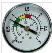
0,8 \text{ kg/cm}^2 : Initial pressure of the filter at the start of a filtering cycle.
