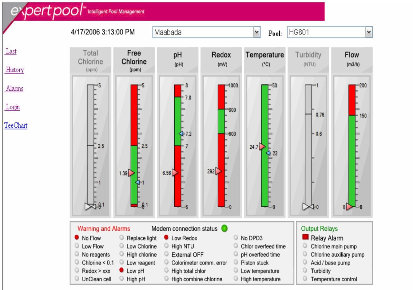
Figure 5: Initial Pool Summary Display: Current Values, Alarms and Relay Operation
