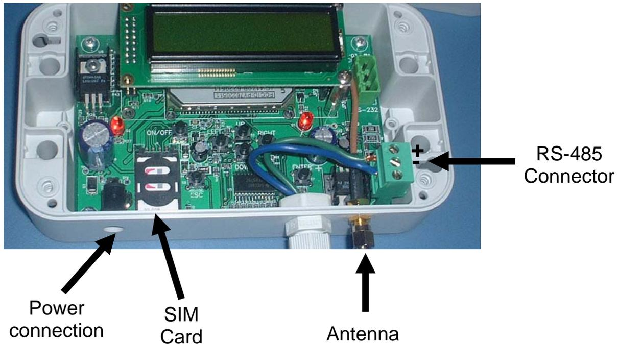
**Figure 2:** Expert Pool Communicator – Internal Components
