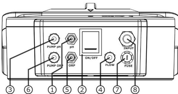
Fig. 4. UV LP/LP+ system control panel. Rear view.
