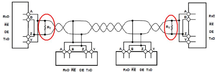
Image 3: terminating resistors
