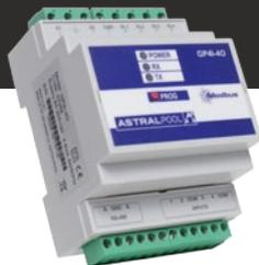
It has 4 digital input and output pins.
