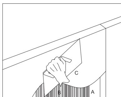
*Ensure that the fibers are flat within the recess (A). Doing so will ease the rendering-over operation.*
