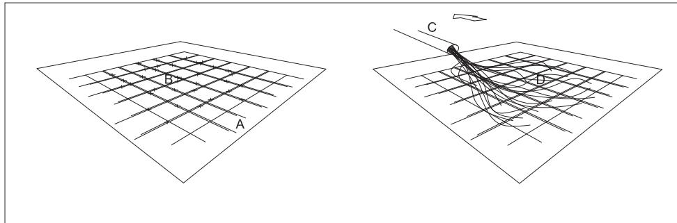
With a chalk line, trace on the surface to be tiled a grid with the spacing and the gaps between tiles (A). Distribute the fiber points in accordance with the chosen design as detailed on 1.0.3 and mark with spray. Ensure that the marks are in the joints between the tiles (B).
