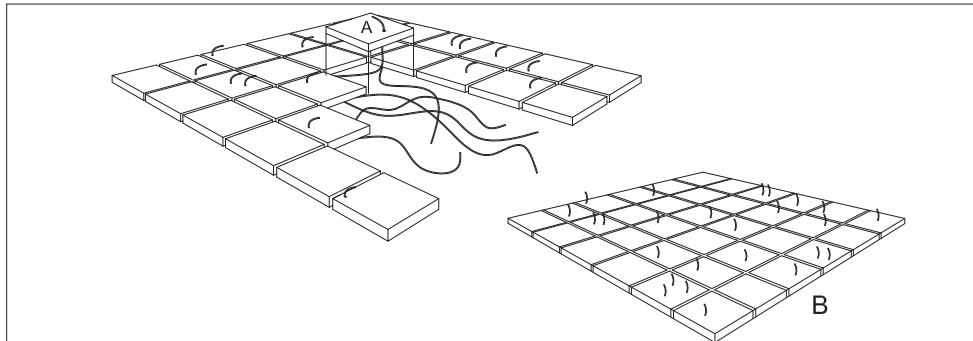
Once the pieces have been drilled through, set tiles in place pulling the fibers through the holes before tampering down, and finish the full surface repeating the previous steps at every fiber point (A).
