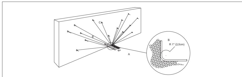
Once the fibers are attached to their respective I1091-0002 supports; render over (A) roughly with a minimum 1/2" (12mm) thickness to hold the fibers/supports in place.
