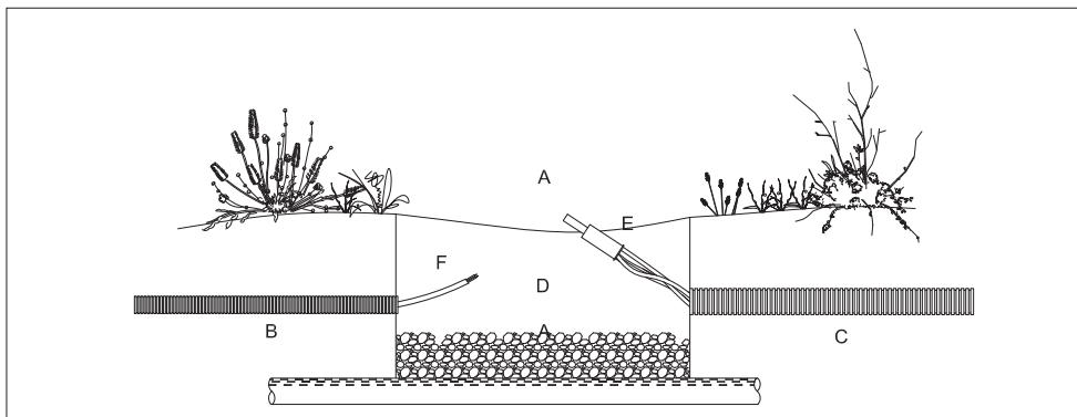
Once the location of the illuminator housing (A) has been determined, lay two conduits or corrugated tube to opposite sides of the housing (D). The conduit (B) should house the 12VAC power cable (F) from the transformer location. Conduit (C) should house the fibers (E) to a point close to the effect installation.
