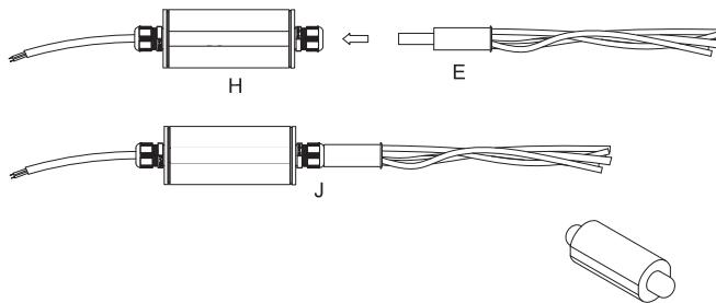
Insert the optical port or fiber connector (E) into the pressure gland in the LED illuminator (H) gently pushing until the connector tip can go no farther.
