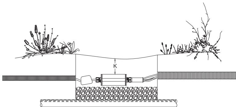
Backfill the housing or trench with a mixture of coarse sand and aggregate or loose gravel, to finish with a layer of garden soil. The illuminator should be at a minimum depth (K) of 200mm from the surface. If the area where the illuminator is buried is walk-over, suitable elements should be placed over to prevent crushing the fibers.
