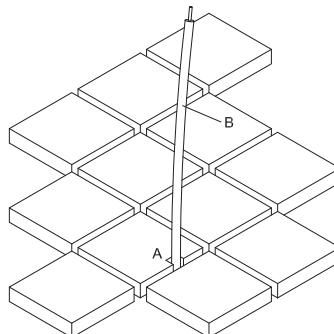
Pour and work well with a squeegee the finishing slurry into the joints (A), ensuring that the notches around the fibers don't have any voids. Clean surplus material, brush and leave to dry overnight. With a sharp blade (B) cut the fibers flush with the surface of the mosaic. Once all fibers are flush with the mosaic skin (C), polish with paste applied with a felt disk.
