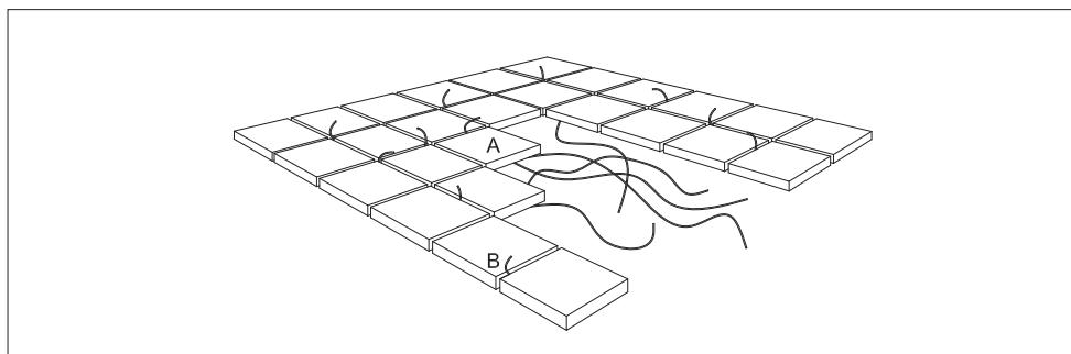
Set tiles in place (A), pulling the fibers through the space in the joints (B) before tampering down and finish the full surface repeating the previous steps at every fiber point.
