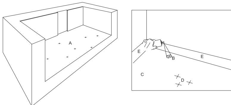
Mark the star pattern on the bottom of the basin with chalk or other erasable medium (A). From outside the pool or a vantage point, assess the overall distribution. For best results, distribute the points on a scale drawing and later transfer the layout to the basin's floor. Once the pattern is finally determined, apply a spot of spray marking paint to render each point's position permanent (B).
