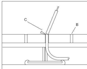
Carefully check over that the fiber points are well set in grout, without any voids. If uneven grout or voids are detected around the fibers, make good with additional grout. Clean in depth the surfaces of the basin (A) using only products without organic solvents. Polish every fiber end with a felt polishing bob (B) attached to a drill, to ensure the points are perfectly flush with the surrounding ceramics.
