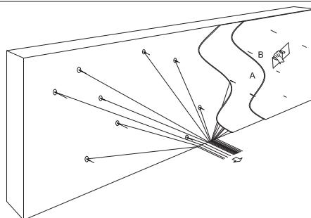
Once the surface is dry (A), apply paint or finish as required. The fibers don't need any protection and can be painted over. The finish must be thoroughly dry (not only surface dry) before attempting to cut the fibers, to avoid paint smudges over the bare ends. Cut the fibers flush with the finish (B) as described on 1.1.3.
