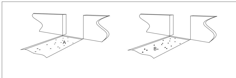
Once the mortar has sufficiently hardened, trim the fibers flush with the wall surface using a sharp (A) blade or the type of pliers used for electronic work. Standard pliers or cutters shouldn't be used; their pyramid jaws squash the fibers before cutting and thus reduce the light intensity.
