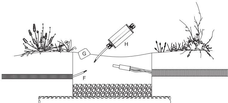
With a suitable connector or connection box (G) join the 12VAC power cable (F) from the remote transformer and the cable from the illuminator (H). The quality of the connection is critical to prevent failures due to moisture penetration. If installed underground, an IP68 connector is mandatory.
