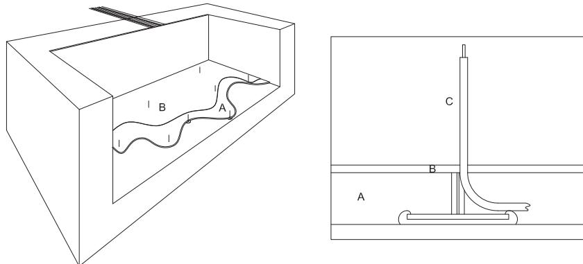
Over the self-leveling screed (A), the craftsman should trowel tile adhesive (B) over a smaller area than usual if the adhesive's curing time is limited. Working on a surface with fiber inclusions is considerably slower than traditional tiling. Great care should be exercised not to accidentally damage the fibers with the sharp edges of the trowel or other leveling tool. Keep the fibers (C) free of adhesive.
