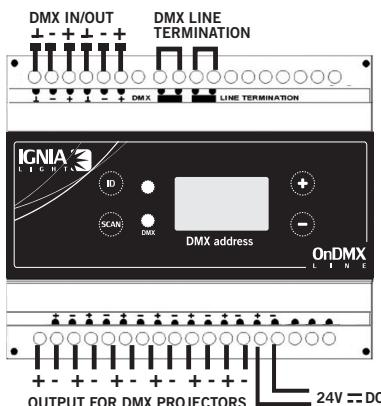
See manual of the DMX mains lead code I0832DMXFE for information regarding how to assing DMX addresses to each projector and how to configure a system.
