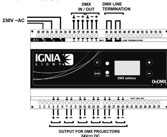
See manual of the DMX mains lead code I0832DMX for information regarding how to assing DMX addresses to each projector and how to configure a system.
